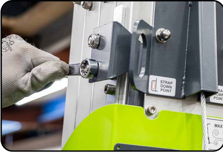
5. Remove both nuts from the top of the mast lock mechanism using a 17mm spanner.
