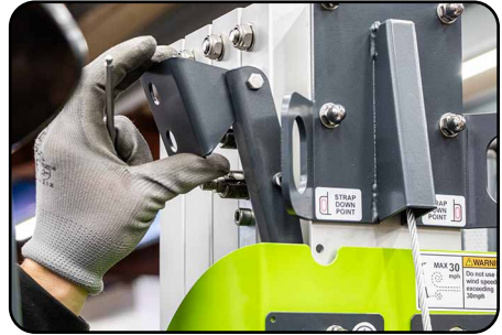
8. Remove the mast lock mechanism handle.
