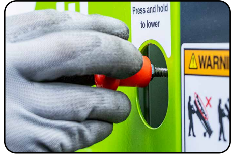
6. Unscrew and remove red mast release knob E.
