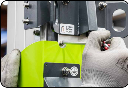
7. Remove the hex bolt directly above the earthing point.
