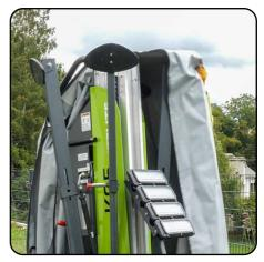
2. Undo the zip. Grab the top of the cover at its edge and lift over the stowed legs on one side of the unit.
