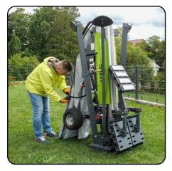
1. Ensure the Quad Pod is fully stowed for transport with the legs raised and light heads stowed in their usual position. Undo the top and bottom straps.
