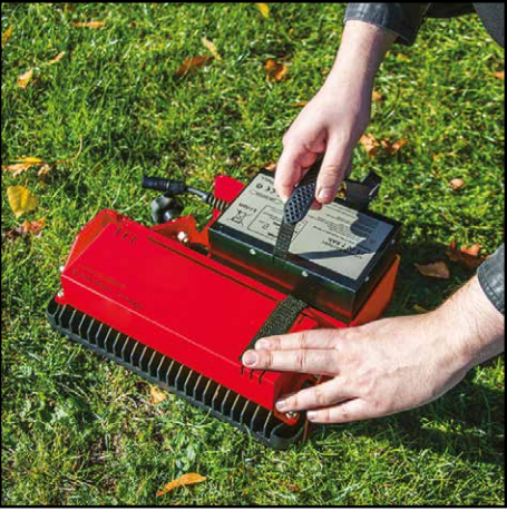
7. Place the battery pack into the bracket. Only use the handle provided to lift the battery, never the battery cable.
