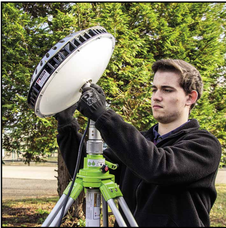
6. Adjust the light heads to point in the required direction by slackening knob 'F', then re-tightening once the desired angle is set.
