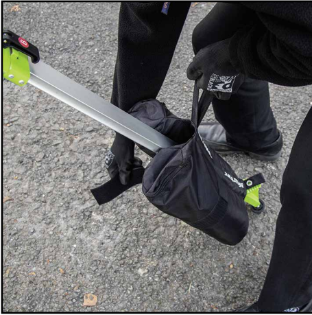
4. If conditions demand it, add sand bags to each leg in the position shown.
