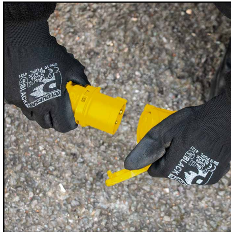
3. Connect the mains input lead to the K21. Observe the local voltage is correct to match the input range of the LED driver (100-277V AC) and switch on / connect power.
