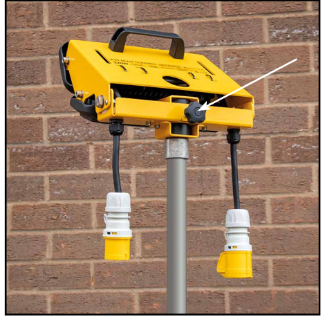
2. Adjust the light head to point in the required direction by slackening knob, then re-tightening once the desired angle is set to prevent it from rotating. If necessary raise light head to required working height.
