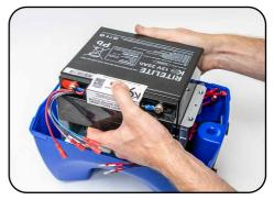
6. Place the replacement battery into the bracket, the same way around as it came out. Take care not to trap your fingers between the battery and bracket.
