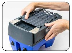
**9.** Carefully fit the grey section of the base fully back onto the blue part of the base checking no cables are obstructing.
