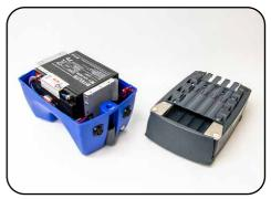
**2.** Lift the grey section from the blue section of the base. If possible keep the bolts and washers in place as this will ease reassembly later.
