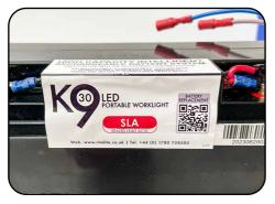
5. Check the new battery has a red lozenge on the label and similar connectors to the one it is replacing.
