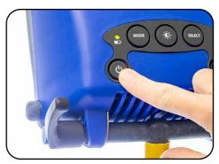
**14.** Test the unit is working correctly by powering on the light head. If working as it should the battery replacement is complete.
