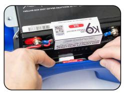
8. Tuck the cables and connectors down the side of the battery bracket, ensure the cables are not twisted or caught by the bracket. Sit the grey base loosely on top. Make sure wires are not caught in between the plastic mouldings.
