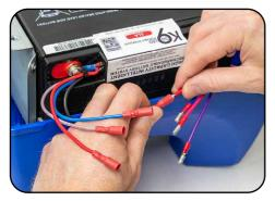
**3**. There are 4 wires alongside the battery. Grip the red connectors on each wire in turn, gently twist and pull them all apart.
