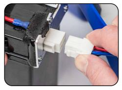
6. Reconnect the battery to the cable connector. The tab should be on the left as shown. Push in until it clicks into place.
