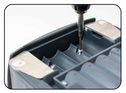
**1.** Remove the light head from the base unit, and turn the unit upside down. Remove the 4 poles from the base. Unscrew the 4 x 4mm hex bolts (2 are located under the pole retainer). DO NOT remove the pole retainer.
