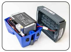
**2.** Lift the grey section from the blue section of the base. If possible keep the bolts and washers in place as this will ease reassembly later. There is a cable attached to the base for the in-built charger, there is no need to disconnect this.
