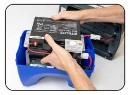
**3**. Carefully lift the battery from the blue base, stand it upright on your work bench next to the blue base. The cable is long enough to allow this.
