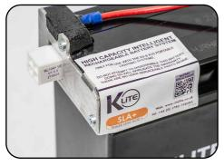
5. Check the new battery has an orange lozenge on the label and the same connector to the one it is replacing.
