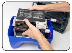
7. Place the replacement battery into the bracket, the same way around as it came out. Take care not to trap your fingers between the battery and bracket.
