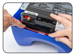
8. Tuck the cable down the side of the battery bracket, ensure the cable is not twisted or caught by the bracket. Sit the grey base loosely on top.
