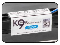
5. Check the new battery has a cyan lozenge on the label and similar connectors to the one it is replacing.
