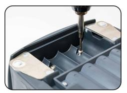
1. Remove the light head from the base unit, and turn the unit upside down. Remove the 4 poles from the base. Unscrew the  $4 \times 4$ mm hex bolts (2 are located under the pole retainer). DO NOT remove the pole retainer.
