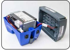
**2.** Lift the grey section from the blue section of the base. If possible keep the bolts and washers in place as this will ease reassembly later. There is a cable attached to the base for the in-built charger, there is no need to disconnect this.
