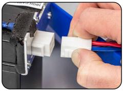
4. You can now get to the battery connector. There is a tab on the side of this, press this in and disconnect the cable.
