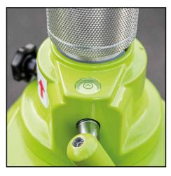
**3.** Observe the in built level and if required adjust legs accordingly as per instruction (2) so the tripod is level and stable.
