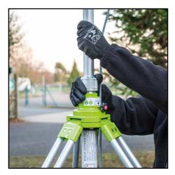
**4.** Next grasp the aluminium section supporting the light heads and undo (D) slowly in an anticlockwise direction until you feel the weight of the light heads as they descend, continue to bear their weight and guide them downwards until they are at a rested position on top of the section below.
