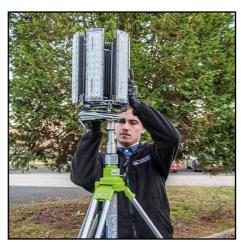
**6.** Coil up any cables attached to the light head. Lift the light head off the unit and place on the ground.
