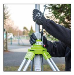
**8.** Unlock the knurled collar (D) in an anti-clockwise direction and extend the mast upwards to the required height (have someone assist if you are unsure of the weight you can manage), then whilst supporting the load tighten the knurled collar in a clockwise direction (D) fully so it is tight and supporting the weight of the light heads safely.
