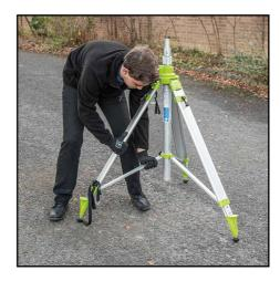
1. Undo the strap which wraps around the tripod legs. Undo the knob marked 'A' on the tripod – fold out legs evenly until the leg tie bars are horizontal to the centre hub point. Tighten knob 'A' to lock off tie bars.
