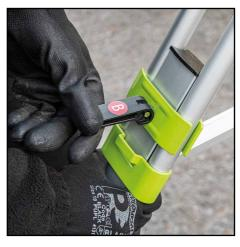
**8.** Support the tripod and then undo each leg locking lever (B) slide each leg up fully in turn and then lock the lever (B) back to retain.
