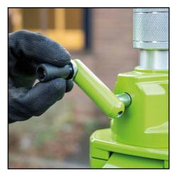
2. Undo anti-clockwise knob (E) and turn the handle anti-clockwise to lower the mast until the next section with the knurled knob (D) comes to rest on the main hub.
