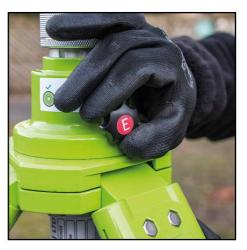
${\bf 10.}$  Lock off knob (E) in a clockwise direction to fully secure mast section.
