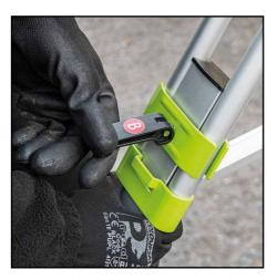
**2.** Extend legs to required height by individually releasing locking lever 'B', extend leg then re-lock lever 'B' making sure it is secure.
