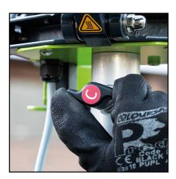
**5.** Slacken off knob of the light head where it attaches to the tripod mount.
