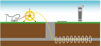
To locate the direction of the non-metalic duct or drain, attach a signal generator to one of the terminals of the Flexitrace and an earth stake (or other independant earth). The Flexitrace can be pushed the length of the duct or drain and then traced along it's complete length with a Cable Avoidance Tool (CAT Receiver).
