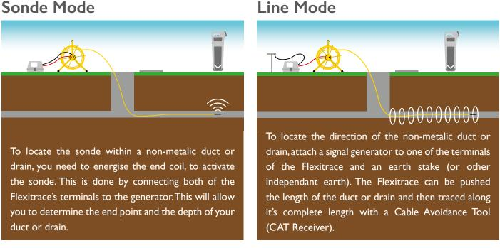
The compact size of the end coil (8.1mm diameter) and the flexibility of the 4.5mm rod make the Flexitrace particularly suitable for locating narrow ducts. Suitable for use with most C.A.T and signal generator systems.
