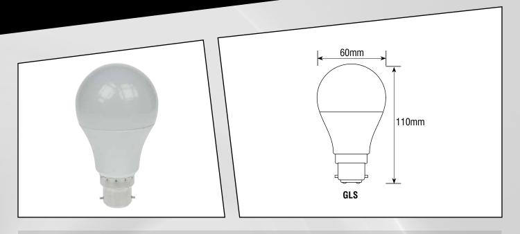
A durable GLS LED lamp with a wide input voltage range of 110-240V made of a shatter resistant polycarbonate dome. It is 8.5W 806 lumens, available in two colour temperatures - warm white 2700K, and daylight white 6400K. It has an average life of 30,000 hours. It is suitable for all applications, either on site in a festoon, retail, domestic and commercial.
